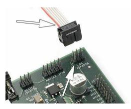
When the AVRISP mkII is connected to both the PC and the target board the main status LED should be green indicating that target power has been detected. AVRISP mkII is now ready to be used with AVR Studio or the programming command line software.
