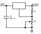
$V_{OUT} = 5V + (5V/R1 + I_0) R2 5V/R1 > 3 I_0$
