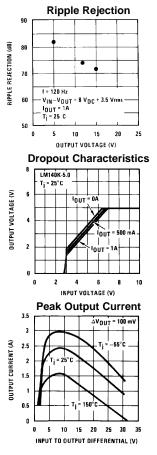
Note: Shaded area refers to LM340A/LM340, LM7805C, LM7812C and LM7815C.
