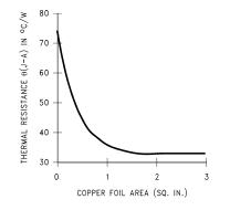
Figure 12.  $\theta_{(J-A)}$  vs Copper (1 ounce) Area for the TO-263 Package
