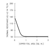
Figure 14.  $\theta_{(J-A)}$  vs Copper (2 ounce) Area for the SOT-223 Package
