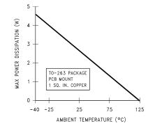
Figure 13. Maximum Power Dissipation vs  $T_{\rm AMB}$  for the TO-263 Package
