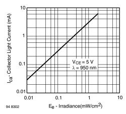
Fig. 4 - Collector Light Current vs. Irradiance
