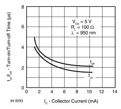
Fig. 7 - Turn-on/Turn-off Time vs. Collector Current
