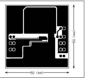
Figure 4. Top view of demonstration board
