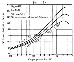
Figure 2. STK4142II Pd – Po ( $R_L = 4\Omega$ )
