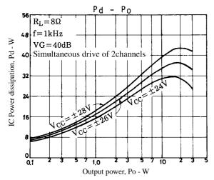
Figure 1. STK4142II Pd – Po ( $R_L = 8\Omega$ )
