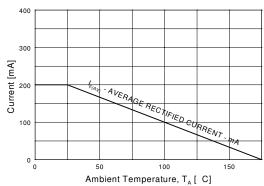
Figure 10. Average Rectified Current ( $I_{F(AV)}$ ) versus Ambient Temperature ( $T_{\Delta}$ )
