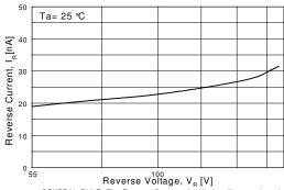
GENERAL RULE: The Reverse Current of a diode will approximately double for every ten (10) Degree C increase in Temperature
