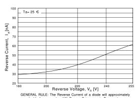
GENERAL RULE: The Reverse Current of a diode will approximately double for every ten (10) Degree C increase in Temperature
