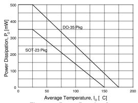
Figure 11. Power Derating Curve
