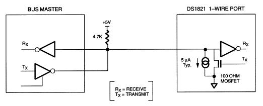
The idle state for the 1-Wire bus is high. If for any reason a transaction needs to be suspended, the bus MUST be left in the idle state if the transaction is to resume. Infinite recovery time can occur between bits so long as the 1-Wire bus is in the inactive (high) state during the recovery period. If this does not occur and the bus is left low for more than 480 µs, all components on the bus will be reset.
