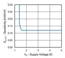
Fig. 13 - Sensitivity vs. Supply Voltage
