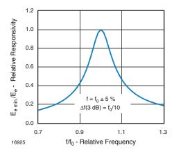
Fig. 5 - Frequency Dependence of Responsivity
