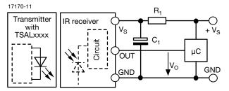
$R_1$  and  $C_1$  recommended to reduce supply ripple for  $V_{\rm S}$  < 2.8 V
