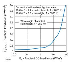
Fig. 6 - Sensitivity in Bright Ambient
