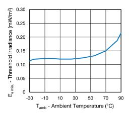
Fig. 9 - Sensitivity vs. Ambient Temperature
