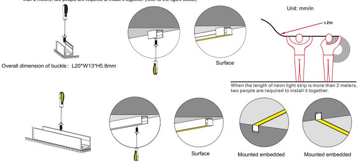
Overall dimension of aluminum profile: L1000\*W13\*H5.8mm
