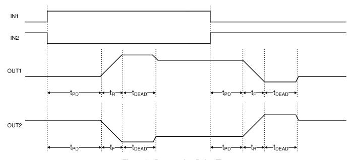
Figure 6. Propagation Delay Time
