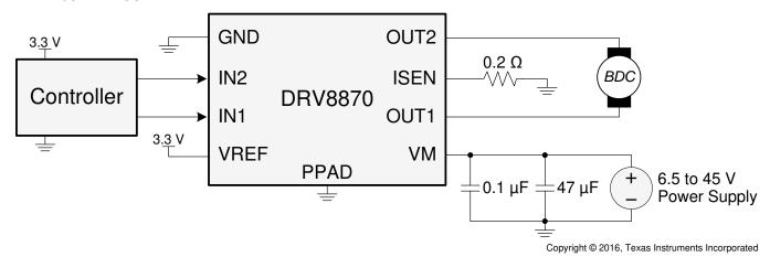
Figure 7. Typical Connections
