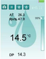
In the Dew Point mode the percentage bargraph indicates how close the IR temperature is to the Dew Point temperature. At 100%, the two values are identical.
