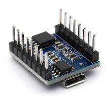
The module contains an MP3 chip that provides a serial port and perfectly integrates hardware decoding of MP3 and WAV. At the same time, the software supports SD card drive, supports direct update of SPI flash content via computer, and supports FAT16, FAT32 file systems. Functions such as playing specified music can be performed with a simple serial port command without the need for cumbersome underlying operations.
