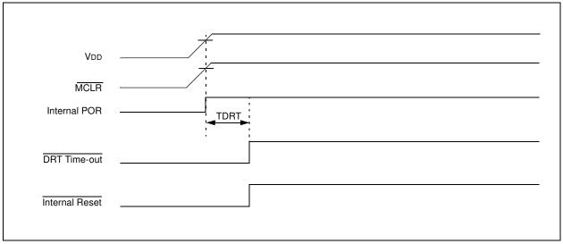
FIGURE 7-11: TIME-OUT SEQUENCE ON POWER-UP (MCLR TIED TO VDD): SLOW VDD RISE TIME
