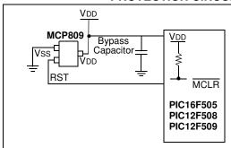
Note: This brown-out protection circuit employs Microchip Technology's MCP809 microcontroller supervisor. There are 7 different trip point selections to accommodate 5V to
