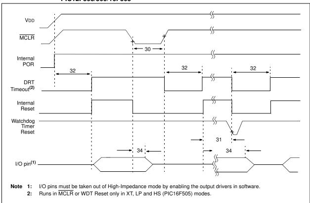
TABLE 10-6: RESET, WATCHDOG TIMER AND DEVICE RESET TIMER – PIC12F508/509/16F505
