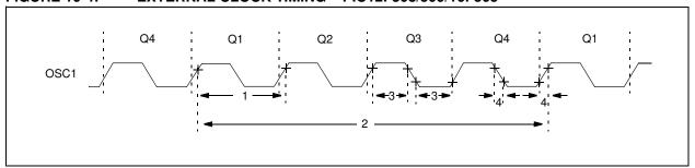
TABLE 10-3: EXTERNAL CLOCK TIMING REQUIREMENTS - PIC12F508/509/16F505
