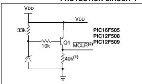
This circuit will activate Reset when VDD goes Note 1: below Vz + 0.7V (where Vz = Zener voltage).
