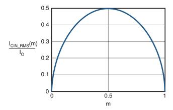
Figure 2. ICIN vs. Voltage Conversion Ratio
