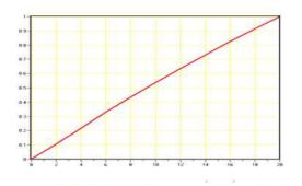
Fig.4 Relative Luminous Intensity-Ta
