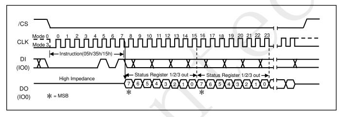
Figure 4. Read Status Register Sequence Diagram
