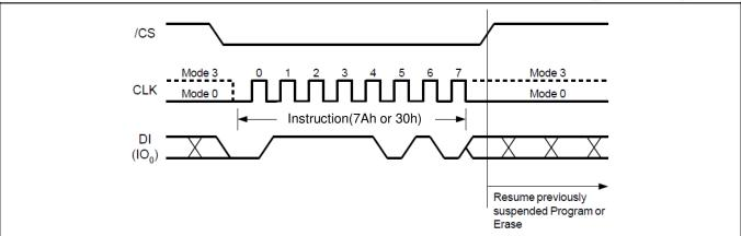
Figure 29. Program/Erase Resume Sequence Diagram
