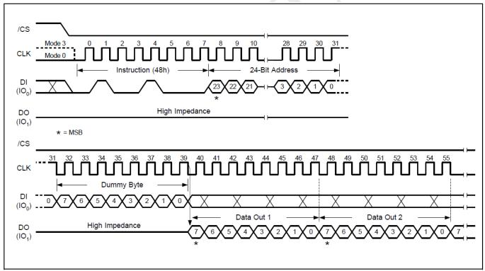
Figure 33. Read Security Registers Instruction (SPI Mode only)
