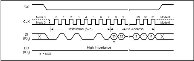
Figure 17. 32KB Block Erase Sequence Diagram
