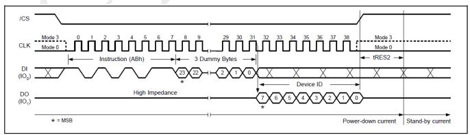
Figure 22. Release Power-Down/Read Device ID Sequence Diagram
