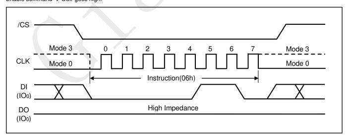
Figure 1 Write Enable Sequence Diagram
