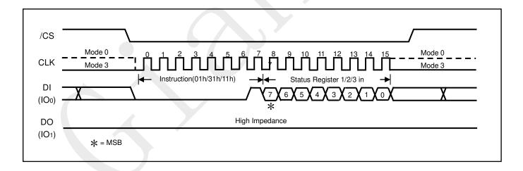
Figure5a. Write Status Register Sequence Diagram
