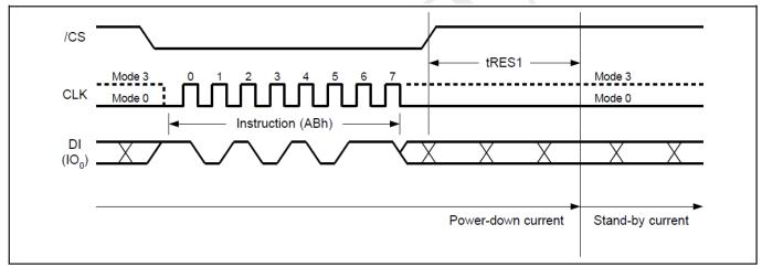
Figure 21. Release Power-Down Sequence Diagram
