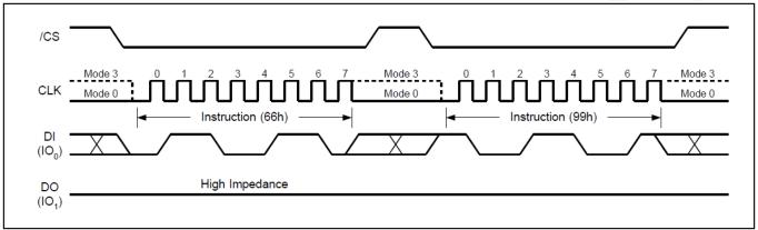
Figure 30. Enable Reset and Reset Instruction Sequence
