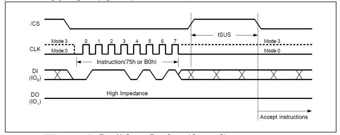
Figure 28. Program/Erase Suspend Sequence Diagram
