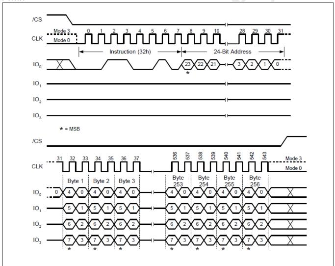
Figure 14 Quad Page Program Sequence Diagram
