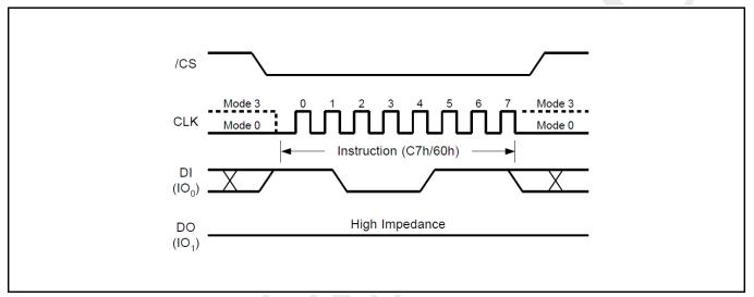
Figure 19. Chip Erase Sequence Diagram
