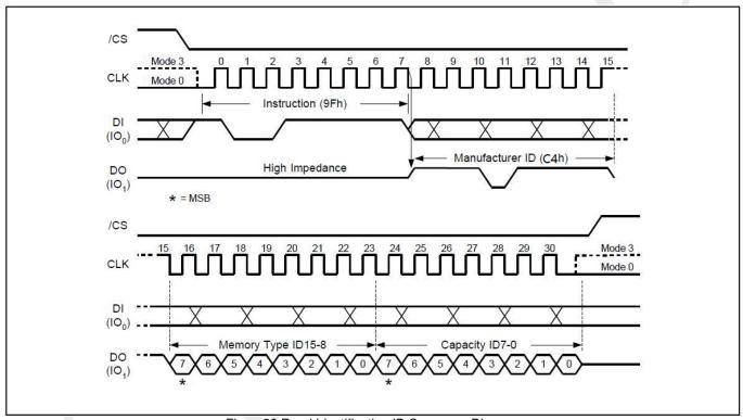
Figure 26. Read Identification ID Sequence Diagram
