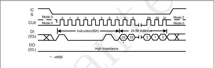
Figure 15. Mini Sector Erase Sequence Diagram
