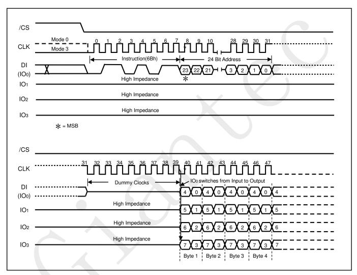
Figure 9. Quad Output Fast Read Sequence Diagram
