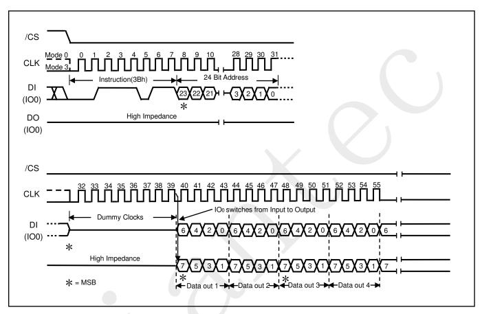
Figure8. Dual Output Fast Read Sequence Diagram
