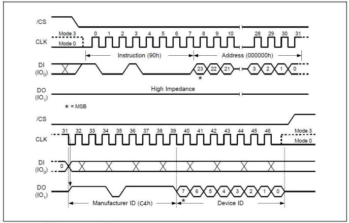
Figure 23 Read Manufacture ID/ Device ID Sequence Diagram
