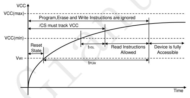
Power-up Timing and Voltage Levels
