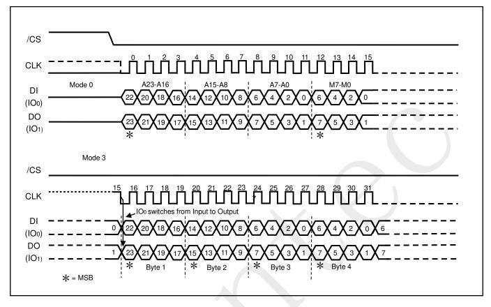
Figure 10a. Duall/O Fast Read Sequence Diagram (M5-4= (1, 0))
