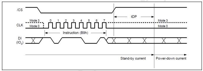
Figure 20. Deep Power-Down Sequence Diagram
