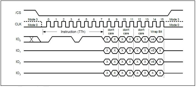
Figure 12 Set Burst with Wrap Sequence Diagram
