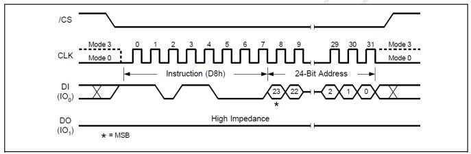
Figure 18. 64KB Block Erase Sequence Diagram
