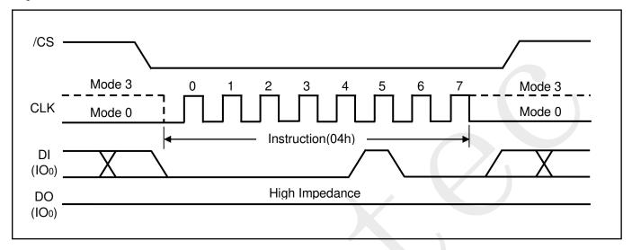
Figure 2. Write Disable Sequence Diagram
