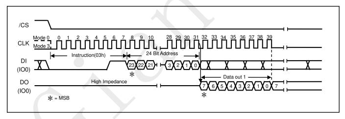
Figure 6. Read Data Bytes Sequence Diagram
