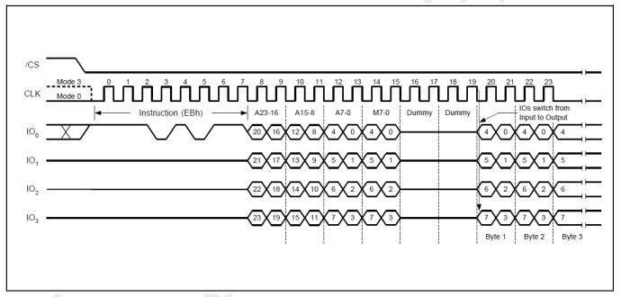
Figure 11. Quad I/O Fast Read Sequence Diagram (M5-4≠(1, 0))
