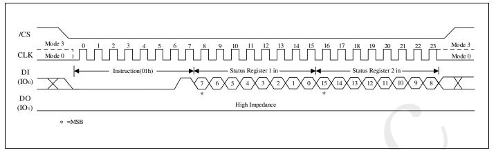
Figure5b. Write Status Register Sequence Diagram
