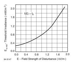
Figure 8. Sensitivity vs. Electric Field Disturbances
