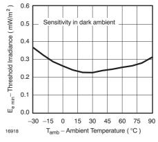
Figure 10. Sensitivity vs. Ambient Temperature
