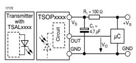
$R_1 + C_1$  recommended to suppress power supply disturbances.
