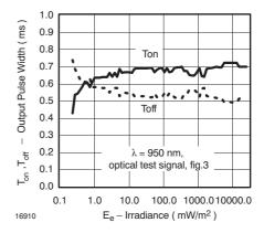
Figure 4. Output Pulse Diagram
