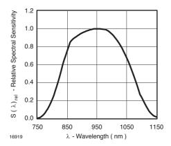
Figure 11. Relative Spectral Sensitivity vs. Wavelength
