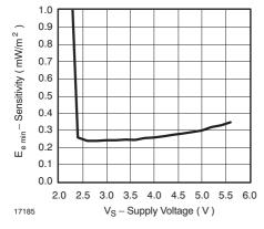
Figure 13. Sensitivity vs. Supply Voltage
