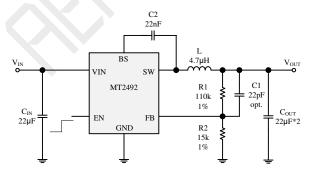
Figure 1. Basic Application Circuit
