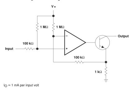
Figure 14. Voltage-Controlled Current Sink
