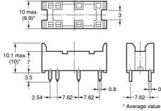
**PCB Mounting Holes** (BOTTOM VIEW)
