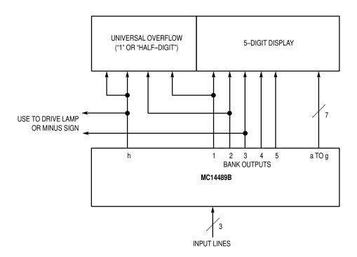
NOTE: A Universal Overflow pins out all anodes and cathodes.
