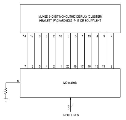
Figure 19. Compact Display System with Three Components
