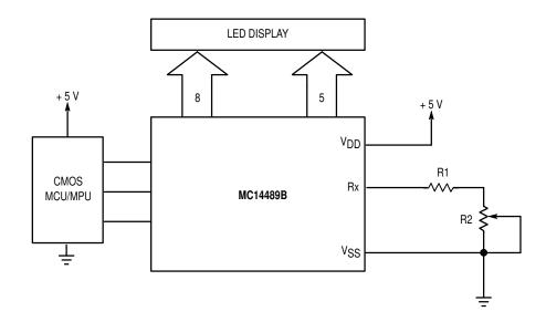
NOTE: R1 limits the maximum current to avoid damaging the display and/or the MC14489B due to overheating. See the Thermal Considerations section. An 1/8 watt resistor may be used for R1. R2 is a 1 k $\Omega$  or 5 k $\Omega$  potentiometer ( $\geq$  1/8 watt). R2 may be a light–sensitive resistor.
