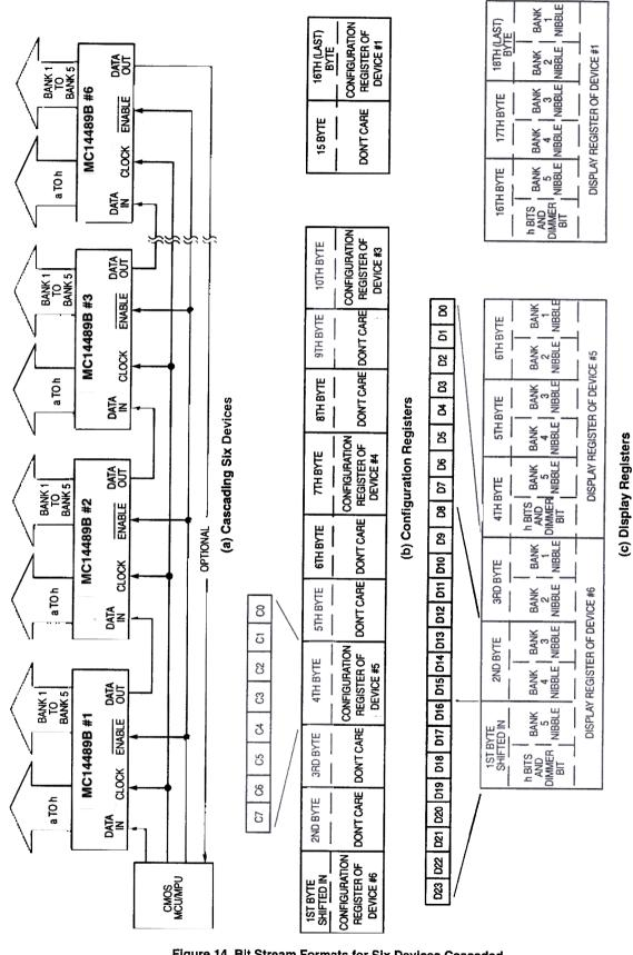
Figure 14. Bit Stream Formats for Six Devices Cascaded
