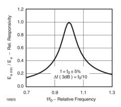
Figure 5. Frequency Dependence of Responsivity
