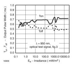
Figure 4. Output Pulse Diagram
