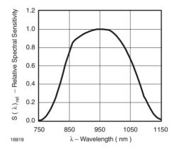
Figure 11. Relative Spectral Sensitivity vs. Wavelength
