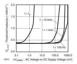
Figure 7. Sensitivity vs. Supply Voltage Disturbances
