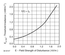
Figure 8. Sensitivity vs. Electric Field Disturbances
