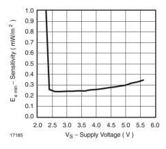
Figure 13. Sensitivity vs. Supply Voltage
