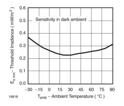
Figure 10. Sensitivity vs. Ambient Temperature
