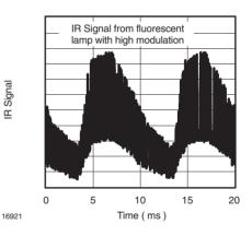
Figure 15. IR Signal from Fluorescent Lamp with high Modulation
