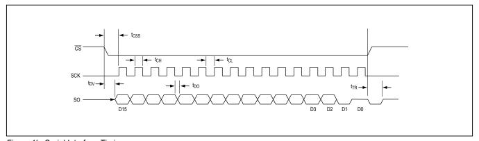
Figure 1b. Serial Interface Timing
