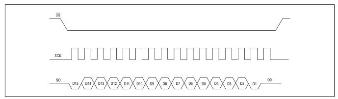
Figure 1a. Serial Interface Protocol
