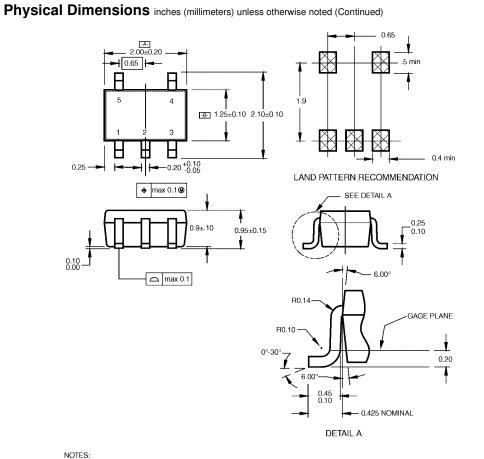
A. CONFORMS TO EIAJ REGISTERED OUTLINE DRAWING SC88A. B. DIMENSIONS DO NOT INCLUDE BURRS OR MOLD FLASH. C. DIMENSIONS ARE IN MILLIMETERS.
