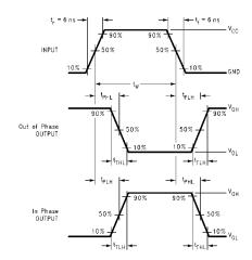
FIGURE 3. AC Waveforms
