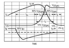
Figure 7. Inductive Switching Measurements
