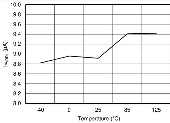
**Figure 1. I<sub>PVDD1</sub> vs Temperature (PVDD1 = 8 V, EN\_GATE = LOW)**
