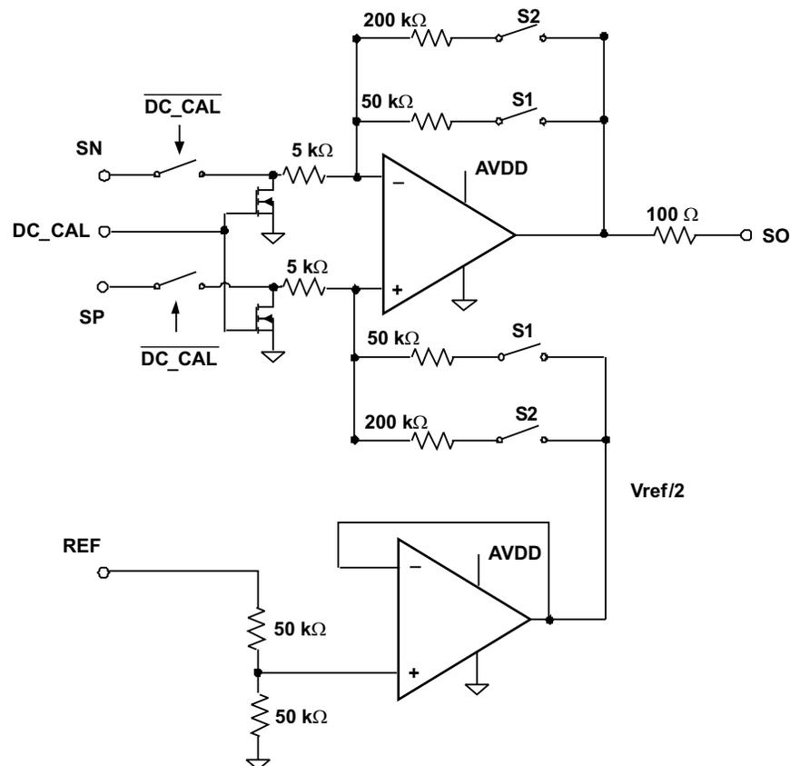
**Figure 4. Current Shunt Amplifier Simplified Block Diagram**
