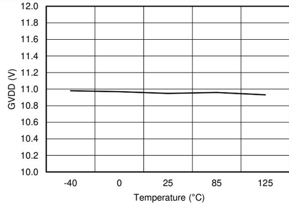
**Figure 2. GVDD vs Temperature (PVDD1 = 8 V, EN\_GATE = HIGH)**
