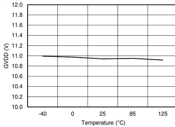
**Figure 3. GVDD vs Temperature (PVDD1 = 60 V, EN\_GATE = HIGH)**
