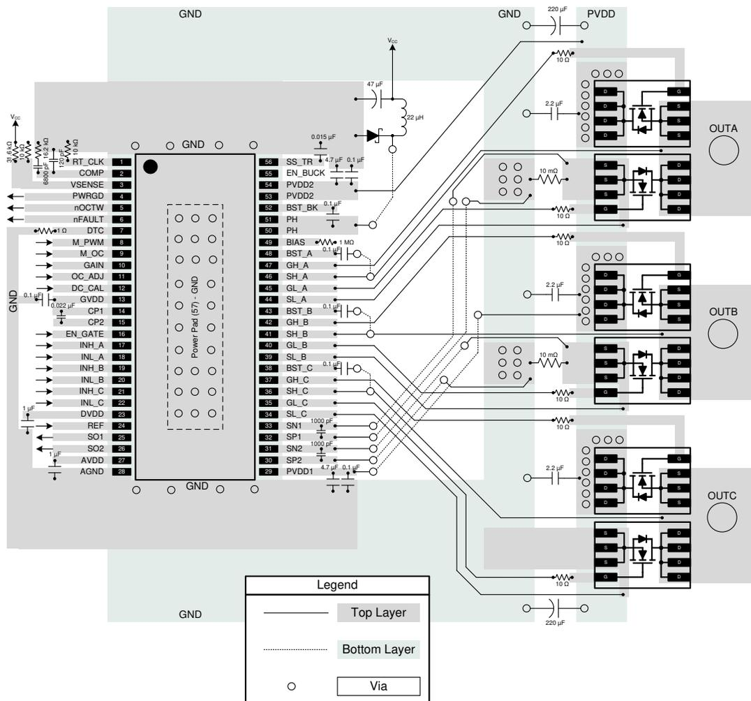
Figure 12. Top and Bottom Layer Layout Schematic
