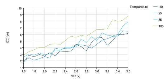
Figure 37-22. Standby Supply Current vs.  $V_{\rm CC}$
