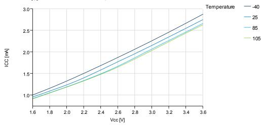
Figure 37-8. Active Mode Supply Current vs.  $V_{\rm CC}$
