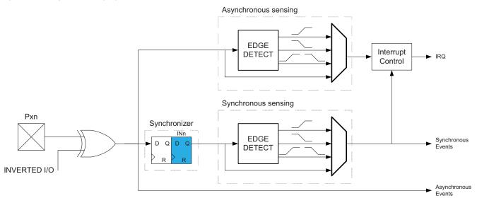
When a pin is configured with inverted I/O, the pin value is inverted before the input sensing.
