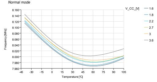
Figure 37-75. 8MHz Internal Oscillator Frequency vs. Temperature
