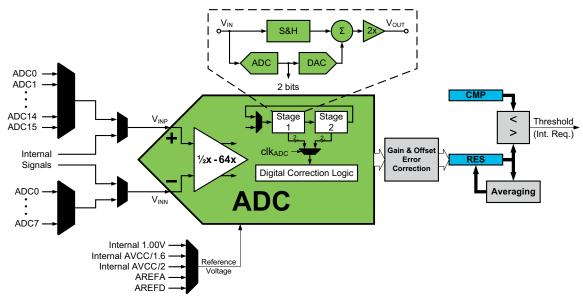
The ADC may be configured for 8- or 12-bit result, reducing the propagation delay from 3.35µs for 12-bit to 2.3µs for 8-bit result. ADC conversion results are provided left- or right adjusted with eases calculation when the result is represented as a signed.
