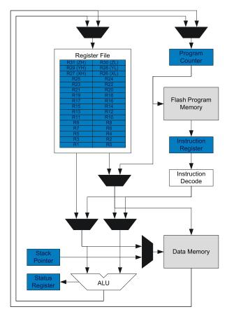
The arithmetic logic unit (ALU) supports arithmetic and logic operations between registers or between a constant and a register. Single-register operations can also be executed in the ALU. After an arithmetic operation, the status register is updated to reflect information about the result of the operation.
