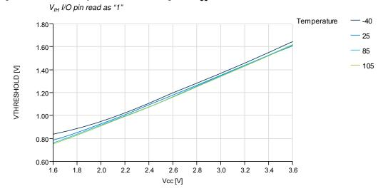
Figure 37-36.I/O Pin Input Threshold Voltage vs.  $V_{\text{CC}}$
