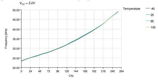
Figure 37-73. 32.768kHz Internal Oscillator Calibration Step Size
