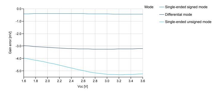
Figure 37-42. ADC Gain Error vs.  $V_{\rm REF}$
