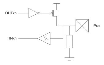
Figure 16-6. I/O Configuration - Wired-AND with Optional Pull-up
