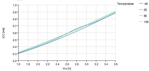
Figure 37-14.Idle Mode Supply Current vs.  $V_{CC}$
