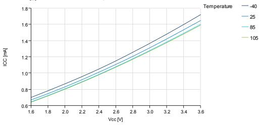
Figure 37-16.Idle Mode Supply Current vs.  $V_{\rm CC}$
