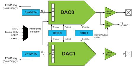
A DAC conversion is automatically started when new data to be converted are available. Events from the event system can also be used to trigger a conversion, and this enables synchronized and timed conversions between the DAC and other peripherals, such as a timer/counter. The EDMA controller can be used to transfer data to the DAC.
