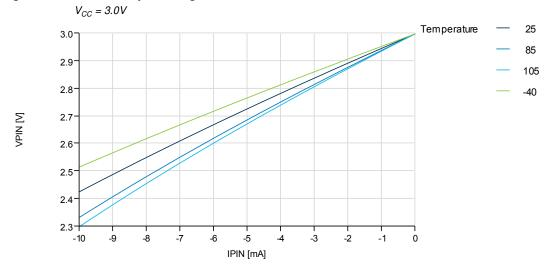
Figure 37-28.I/O Pin Output Voltage vs. Source Current
