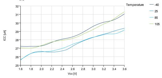
Figure 37-12.Idle Mode Supply Current vs.  $V_{\rm CC}$
