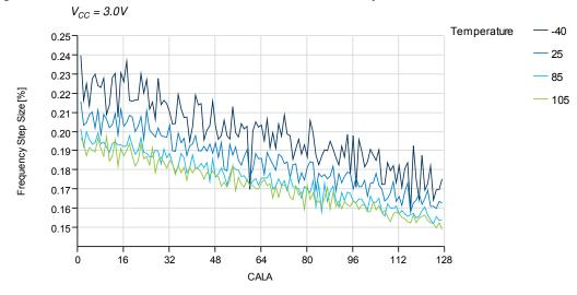
Figure 37-81. 32MHz Internal Oscillator Frequency vs. CALA Calibration Value
