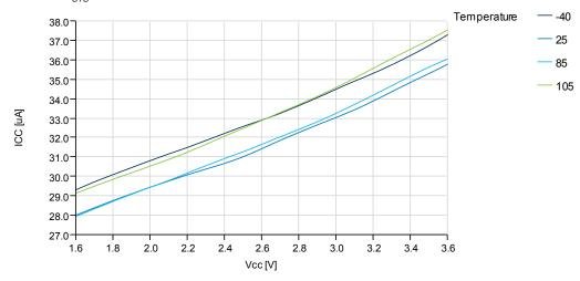
Figure 37-4. Active Mode Supply Current vs.  $V_{\rm CC}$
