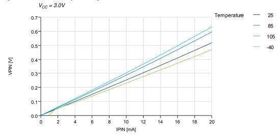
Figure 37-32.I/O Pin Output Voltage vs. Sink Current
