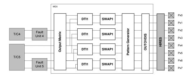
The output matrix (OTMX) can distribute and route out the waveform outputs from timer/counter 4 and 5 across the port pins in different configurations, each optimized for different application types. The dead time insertion (DTI) unit splits the four lower OTMX outputs into a two non-overlapping signals, the non-inverted low side (LS) and inverted high side (HS) of the waveform output with optional dead-time insertion between LS and HS switching.
