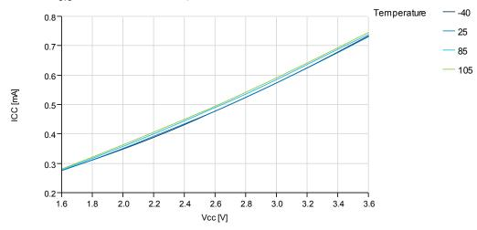
Figure 37-6. Active Mode Supply Current vs.  $V_{\rm CC}$
