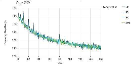
Figure 37-77. 8MHz Internal Oscillator Frequency vs. Calibration
