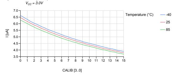
Figure 37-58. Analog Comparator Source vs. Calibration Value
