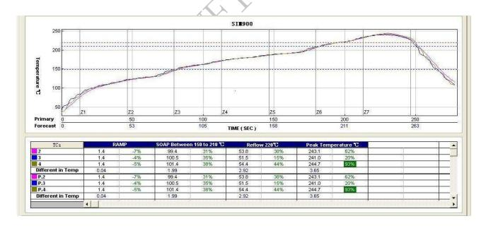
Figure 39: Typical Solder Reflow Profile
