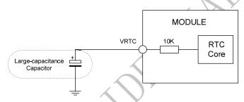
Figure 14: RTC supply from capacitor
