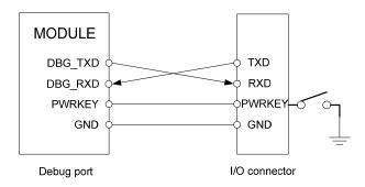
Figure 20: Connection for software upgrading and debugging
