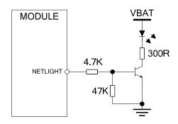
Figure 34: Reference circuit of NETLIGHT
