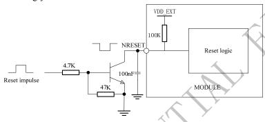
Figure 36: Reset reference design circuit
