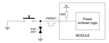
Figure 10: Powered on/down module using button
