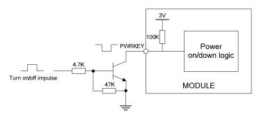
Figure 9: Powered on/down module using transistor
