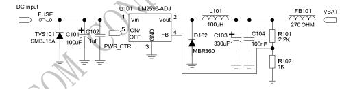
Figure 6: Reference circuit of the DC-DC power supply
