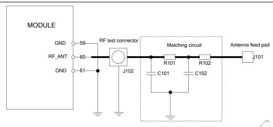
Figure 37: Antenna matching circuit
