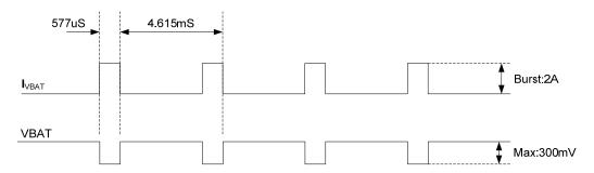
Figure 7: VBAT voltage drop during transmit burst
