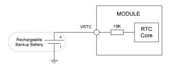
Figure 16: RTC supply from rechargeable battery
