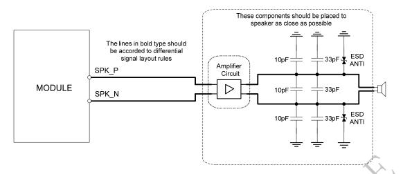
Figure 22: Speaker with amplifier reference circuit
