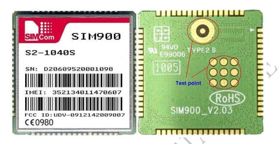
Figure 38: Top and bottom view of SIM900
