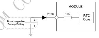
Figure 15: RTC supply from non-chargeable battery
