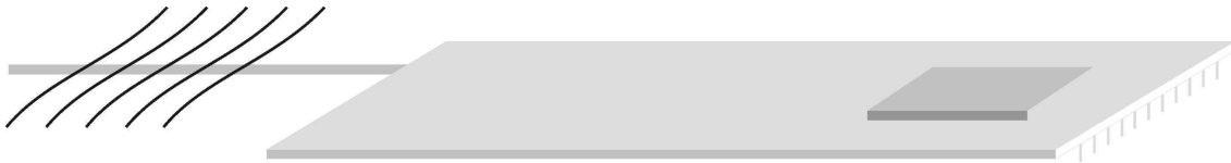
Figure 1 - Antenna area (marked by diagonal lines)
