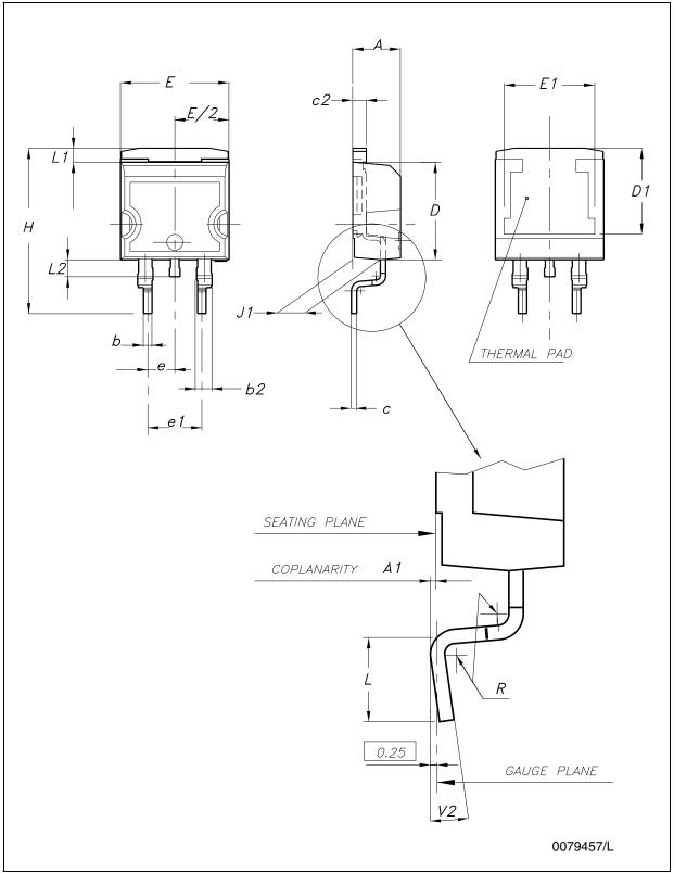
Figure 16. Drawing dimension D<sup>2</sup>PAK (type STD-ST)
