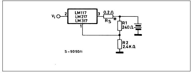
\*  $R_S$  sets output impedance of charger  $Z_O = R_S (1 + R_2/R_1)$ . Use of  $R_S$  allows low charging rates whit fully charged battery.
