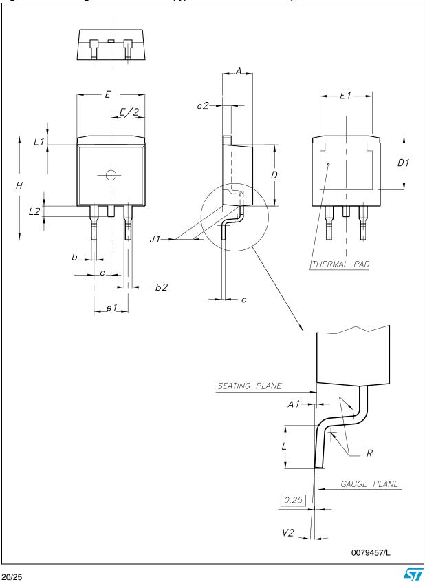
Figure 17. Drawing dimension D<sup>2</sup>PAK (type WOOSEOK-SUBCON.)
