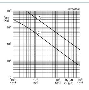
$C_t$  curve at  $R_t$  = 100 k $\!\Omega;~R2$  = 470 k $\!\Omega.$
