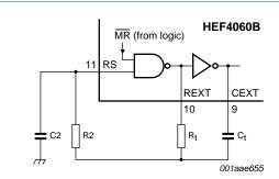
Typical formula for oscillator frequency:  $f_{osc} = \frac{1}{2.3 \times R_t \times C_t}$
