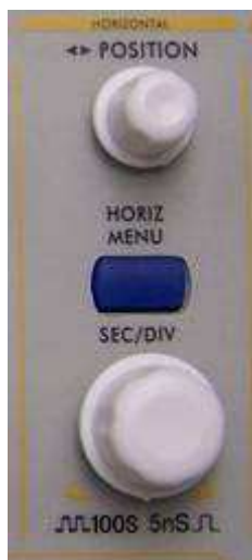
Fig. 10 Horizontal Control Zone
