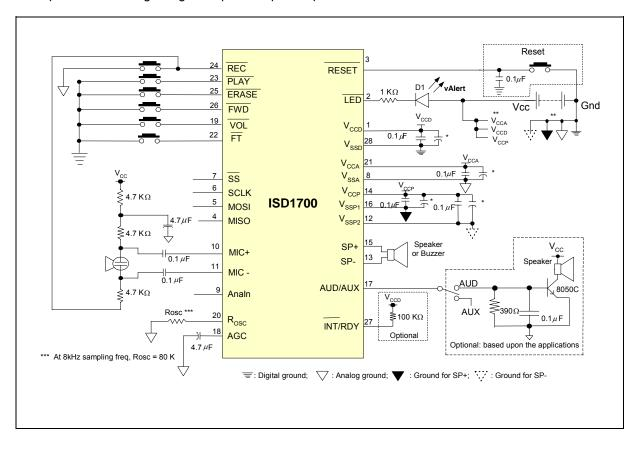
Example #1: Recording using microphone input via push-button controls
