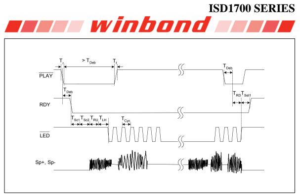
Figure 12.2: Start and Stop Playback Operation
