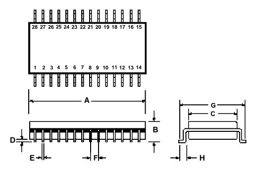
Plastic Small Outline Integrated Circuit (SOIC) Dimensions
