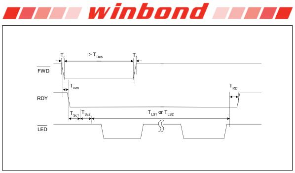
Figure 12.4: Forward Operation with No Sound Effect
