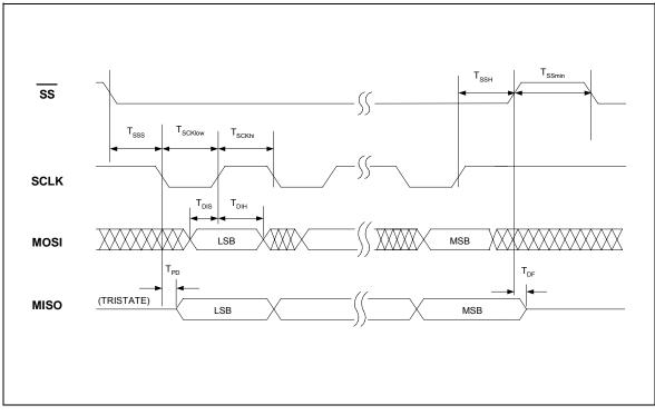
Figure 12.8: SPI Operation
